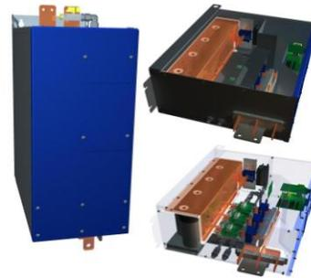
Fig. 3: Sample of design solutions of the power inverter for the solar plants. The first appearance of the inverter is shown in the basic position. On the other illustrations, there are several views inside the inverter.
