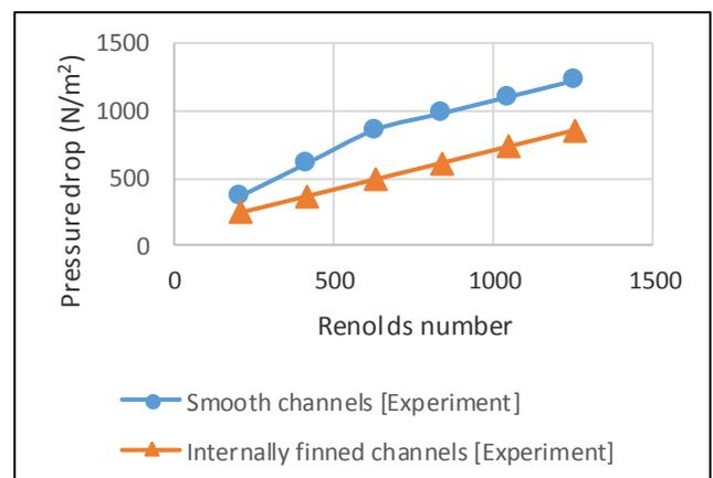
**Fig 3: Pressure drop versus Reynolds number**
