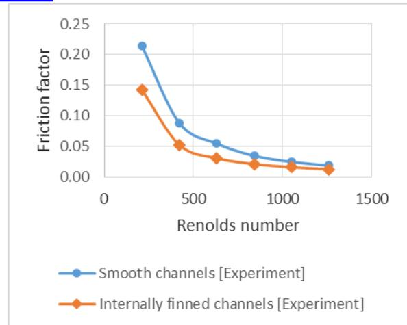
Fig 4: Friction factor versus Reynolds number
