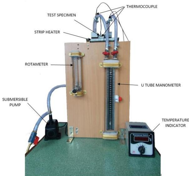
**Fig 2: Pictorial view of experimental test set-up for heat sink**
