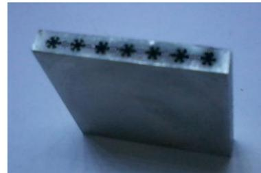
Fig 1: Pictorial view of internally finned channels heat sink
