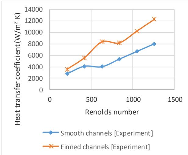
Fig 5: Heat transfer coefficient versus Reynolds number
