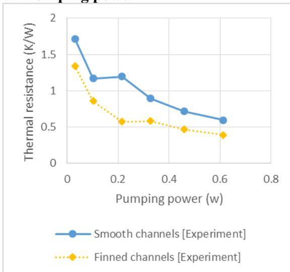
Fig 7: Thermal resistance of heat sink as function of pumping power
