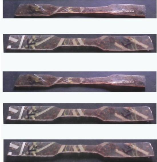
Fig – 3 Before tensile test material
