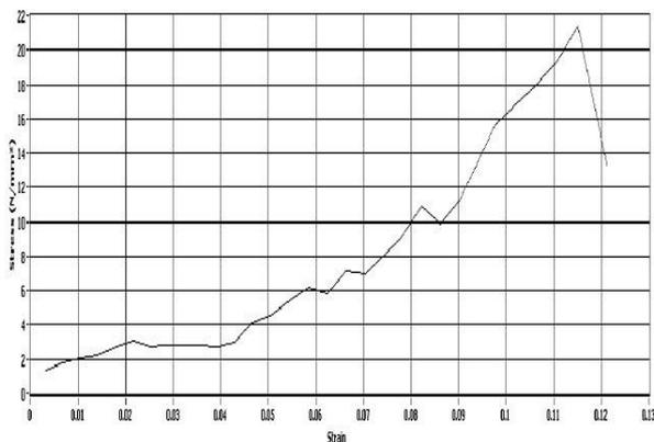
Fig – 9 Maximum Flexural load for Rubber:bamboo=3:7
