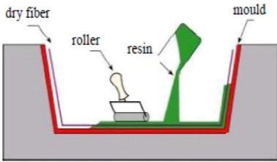
Fig -1 Hand lay up method
