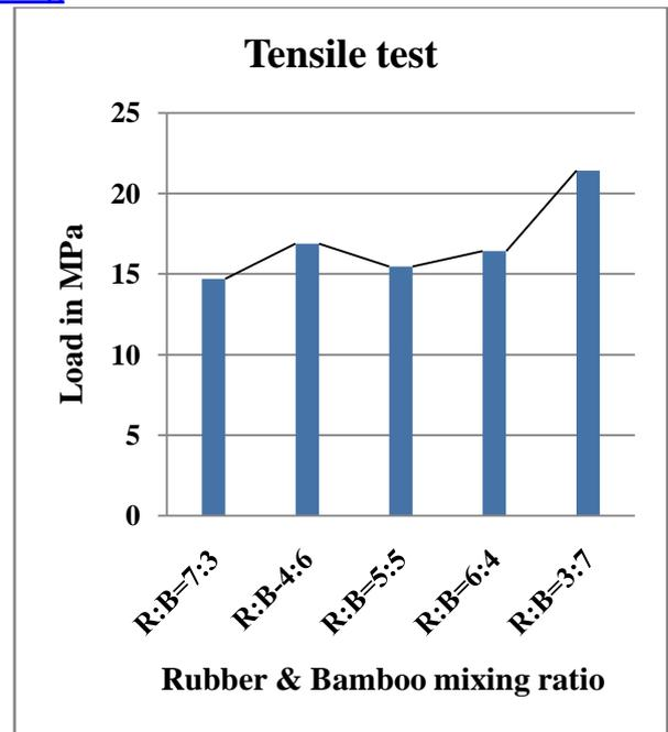
Fig – 6 Tensile test chart (Mpa)
