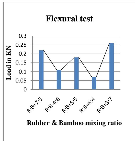
Fig – 7 Flexural test chart (KN)
