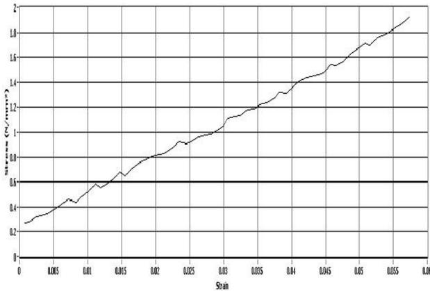
Fig – 8 Maximum tesile strength for Rubber:bamboo=3:7
