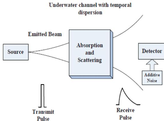
Fig.1. System model of the UWOC link
