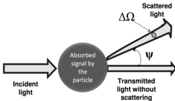
Fig. 2. Light scattering when encountering a particle in water.
