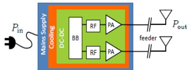
Fig 4. Block diagram of a base station transceiver
