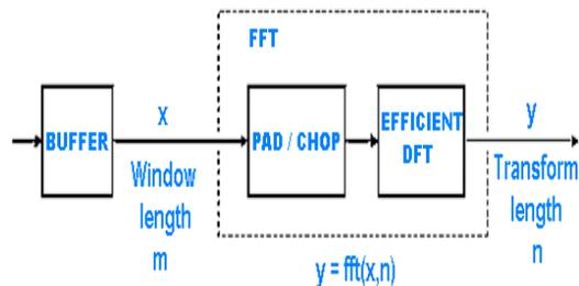
Fig.7 Block Diagram of FFT
