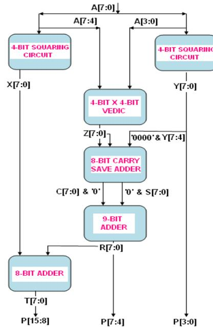
**Fig.5 Architecture of 8-bit Vedic squaring circuit**
