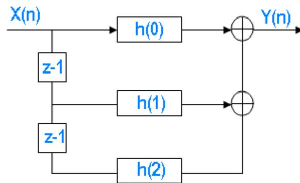
**Fig.6 FIR filter using poly-phase structure**
