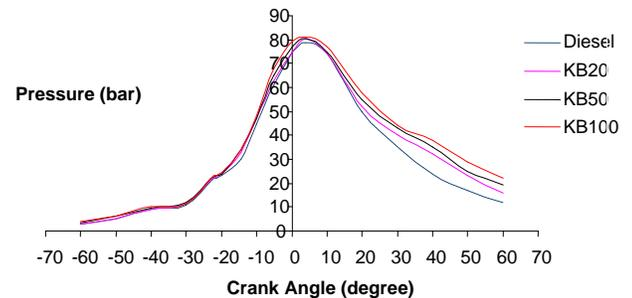
Fig.9: Pressure vs Crank Angle diagrams for Diesel, Karanja biodiesel and blends at full load
