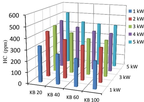
Fig. 8: HC Emission VS Brake Power and % Composition of Blends
