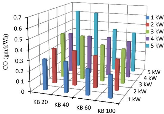
Fig. 7: CO Emission VS Brake Power and % Composition of Blends
