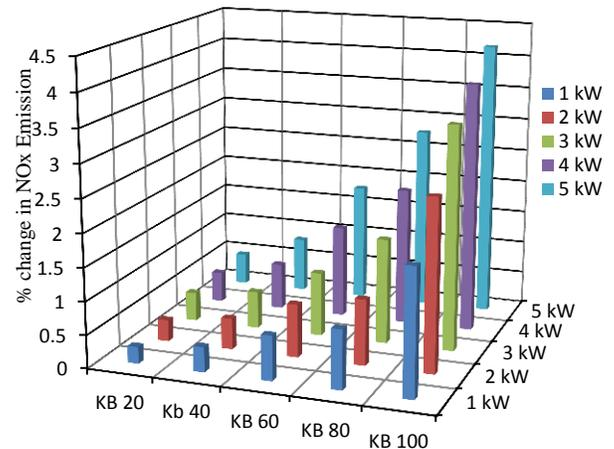
Fig.5. % Change in NO<sub>x</sub> Emission vs Brake Power and % Composition of Blends
