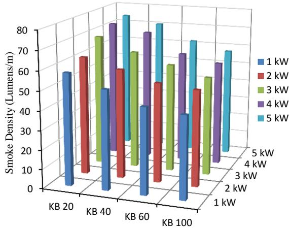
Fig.6: Smoke Density VS Brake Power and % Composition of Blends
