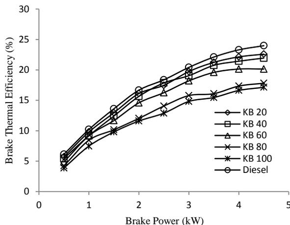
Fig.4. Brake Thermal Efficiency VS Brake Power
