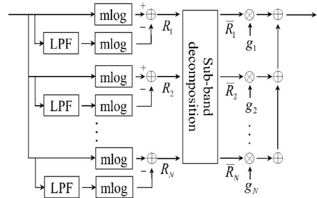
fig1: block diagram of SD-MSR
