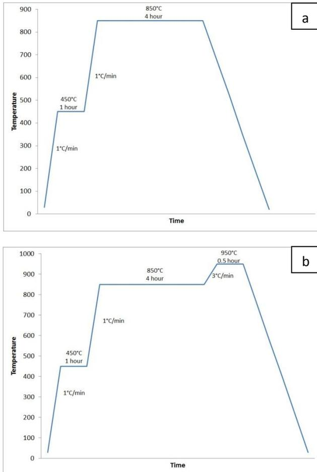
Fig. 2. Two types of sintering schedules to fabricate Cu foam which are (a) 450-850°C and (b) 450-850-950°C.
