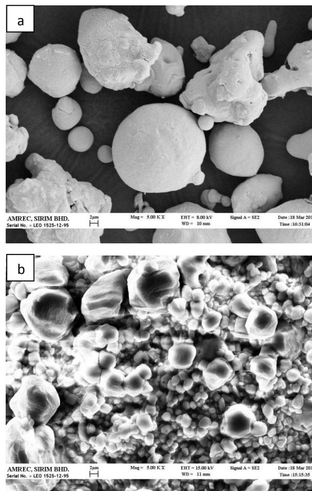
**Fig. 1. Morphology of (a) copper and (b) potassium carbonate powders**
