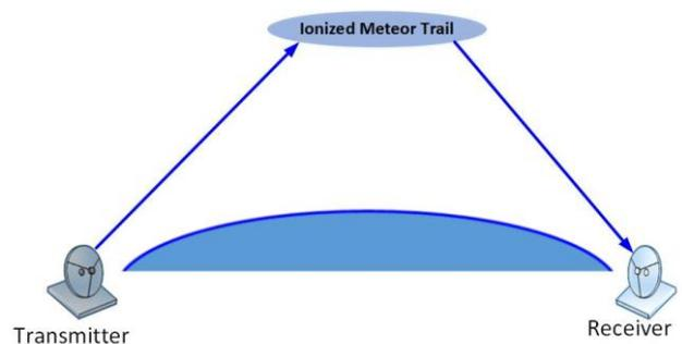
Figure (1) Reflection of radio wave off ionized meteor trail
