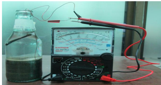
Figure 3: Working scheme of the laboratory scale of the SMFC
