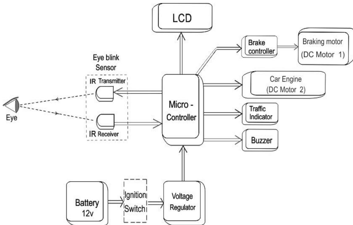
Figure 1 : Block diagram of the vehicle accident prevention system
