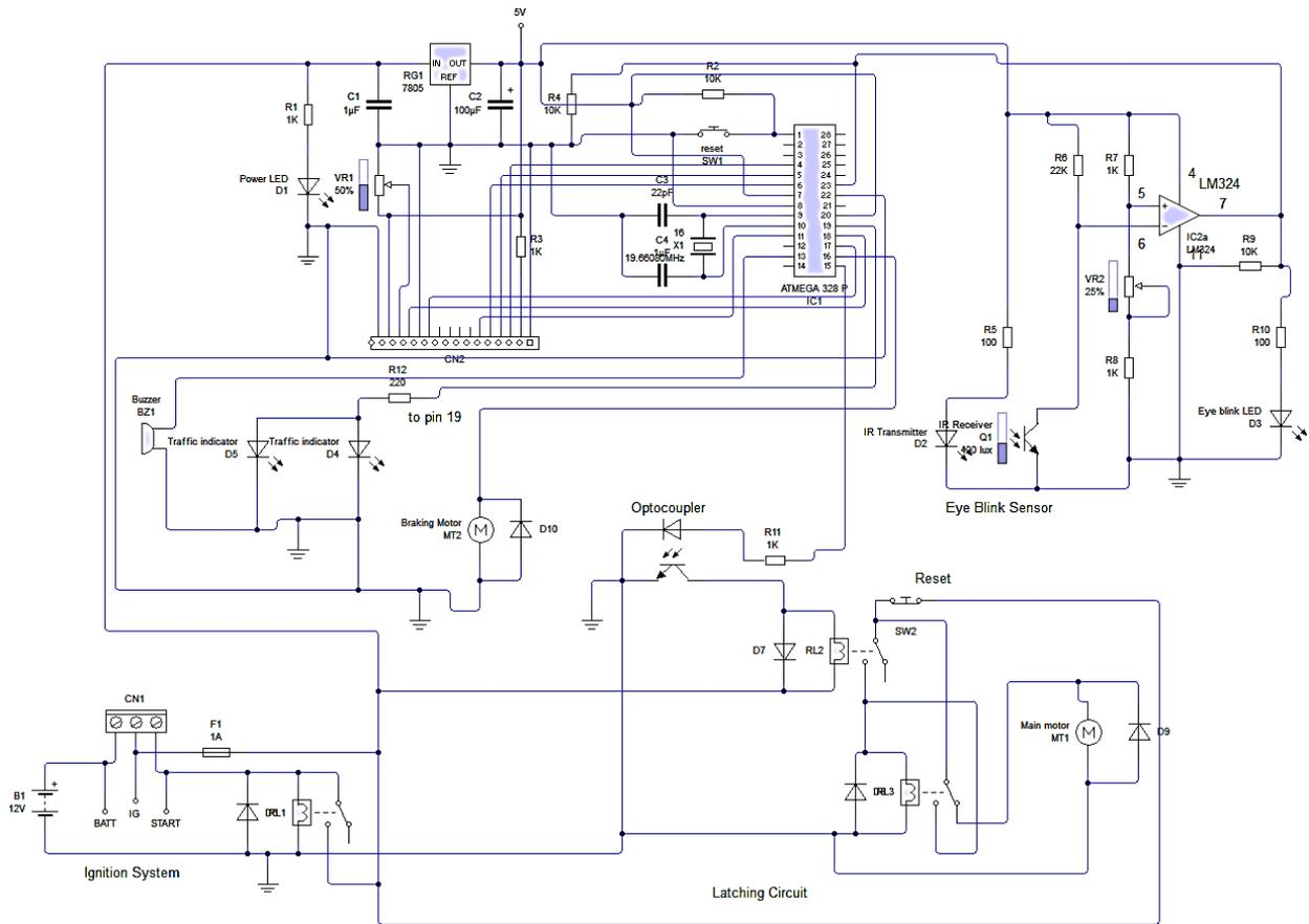
Figure 3 : Circuit Diagram for Vehicle Accident prevention system
