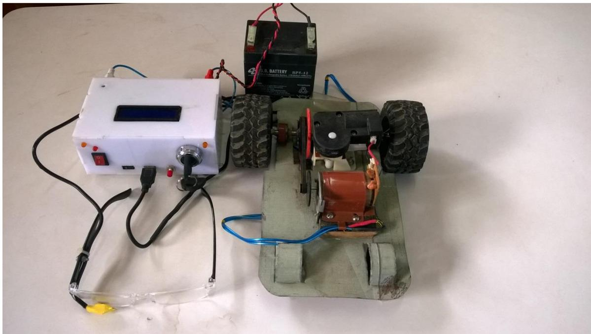
The picture above shows the final construction of the vehicle accident prevention system using eye blink sensor with an automatic braking system.
