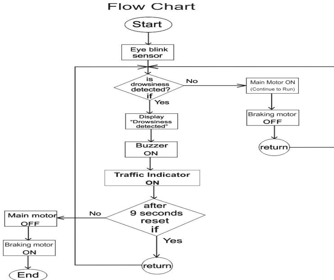
Figure 2 : The Logical Flow (Flow Chart) Model of Vehicle Accident prevention circuit Using Eye Blink Sensor
