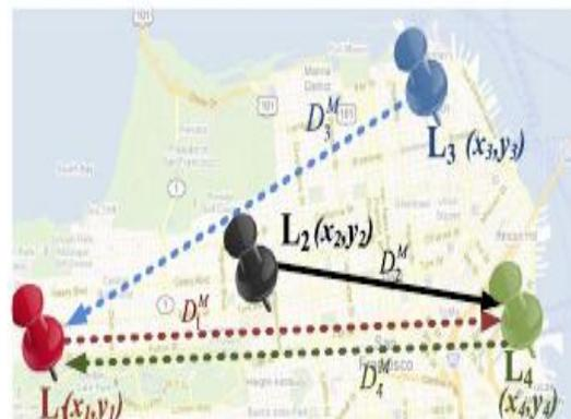
This figure shows a functional diagram of the PFRVP protocol, where the PFRVP algorithm is executed by location determination server. The fairness function  $g$  can be defined in several ways, depending on the preferences of users or policies. The graph shows one such fairness function that minimizes the maximum displacement of any user to all other locations. This fairness function is globally fair and can be easily extended to include additional constraints and the parameters.
