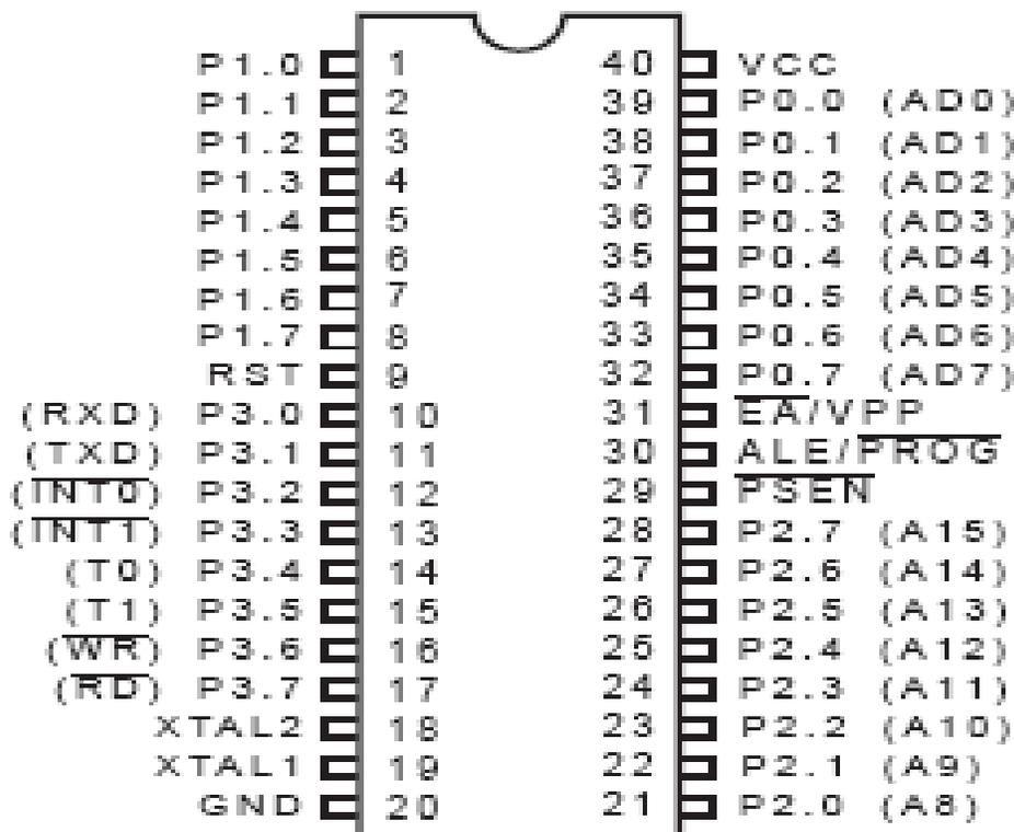
Figure 5: Pin connection of AT89C51 Microcontroller
