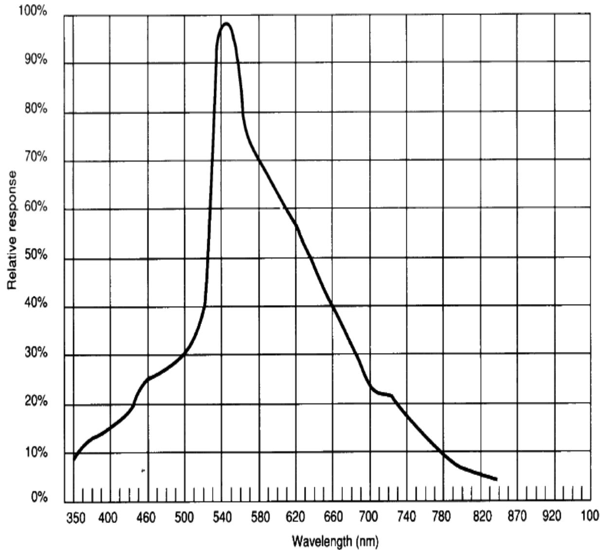
**Figure 8: Spectral Response (Relative Response against wavelength)**
