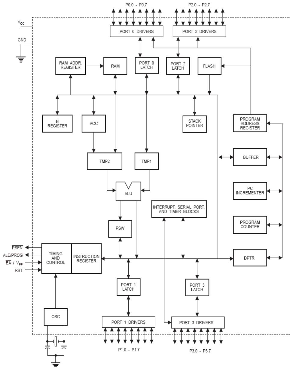
**Figure 5 : Block Diagram of AT89S52 Microcontroller**
