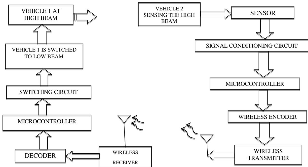
Figure 2: Block Diagram for System Device
