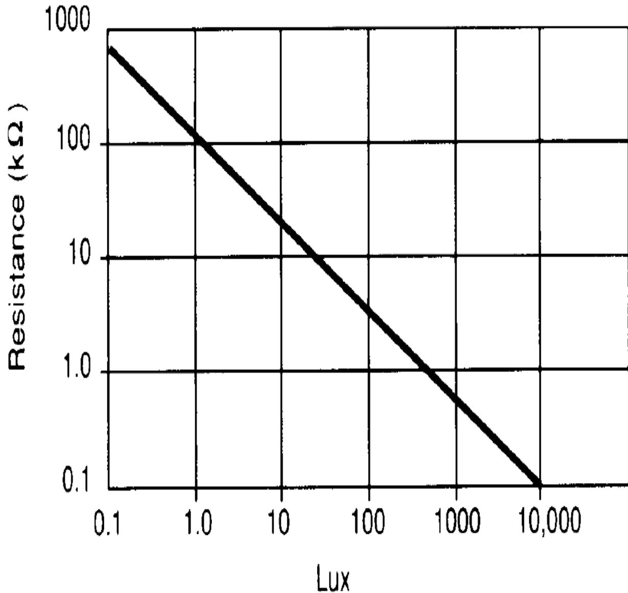
Figure 7: A graph of Resistance against Lux
