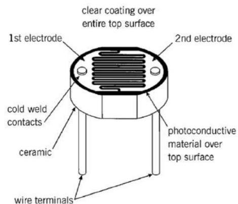
LDR is employed in the circuit to convert the intensity of the high beam headlight of the approaching vehicle into electrical signal. The advantages of LDRs are as follows: they are cheap and are readily available in many sizes and shapes, practical LDRs are available in variety of sizes and package styles, the most popular size having a face diameter of roughly 10mm and finally they need very small power and voltage for their operations.
