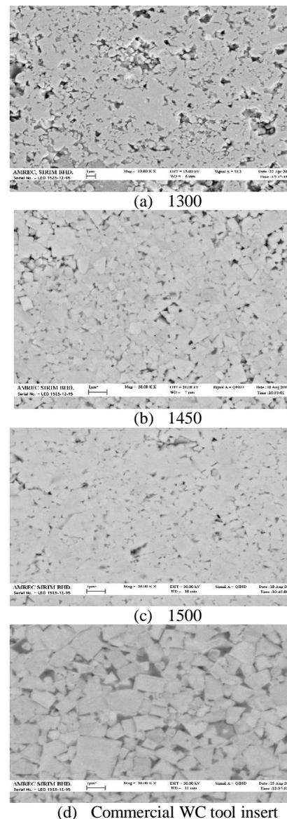
**Fig. 3. SEM micrographs of sintered samples showing the change in WC grain size and morphology at given sintering temperature (a) – (c); and (d) commercial uncoated WC cutting tool insert**
