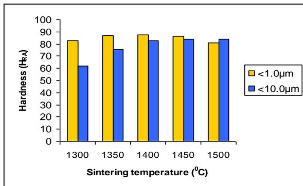
Fig. 4. The relationship between hardness particle size 1.0 µm and 10.0µm of WC at various sintering temperature.
