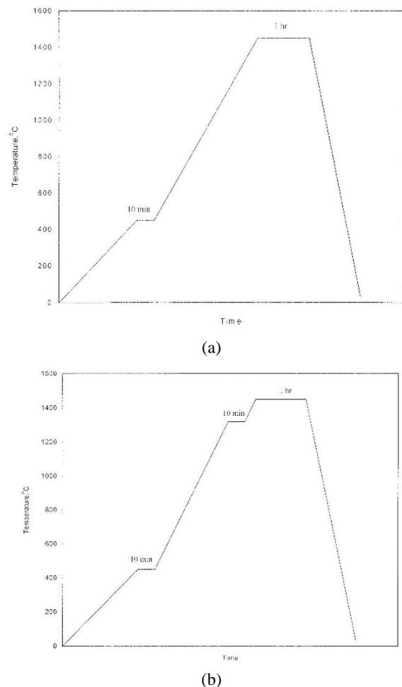
**Fig. 1. Heating schedule for WC-6Co powders compacted at 590MPa; (a) 450-1450°C and (b) 450-1320-1450°C, 1h holding time**
