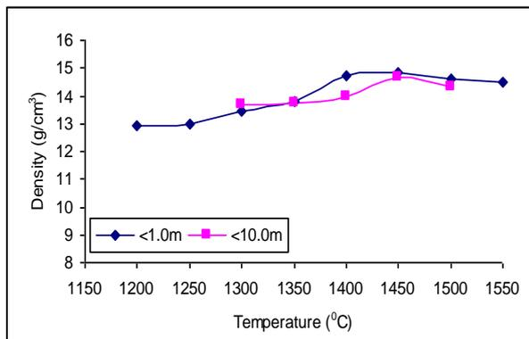
**Fig. 2. The experimental result on the relationship between density of sintered WC-6Co and sintering temperature.**
