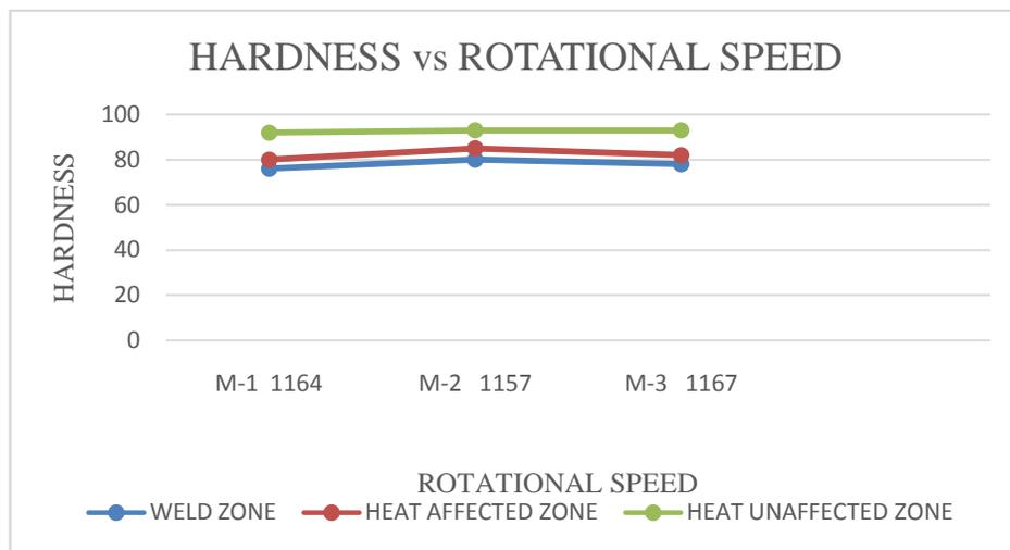
Hardness measured values at different zones for different feeds as given below:
