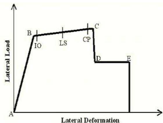
Fig 1: Lateral load versus deformation
