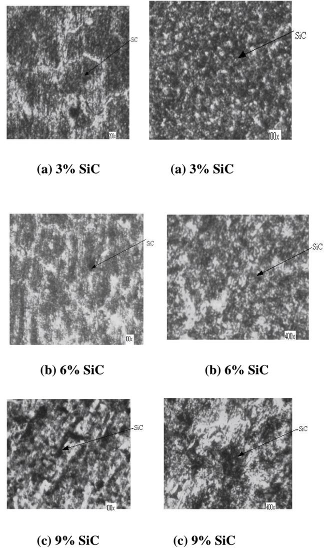
**Fig 3.1 (b) Homogeneous distribution of casting Al7075/SiC**
