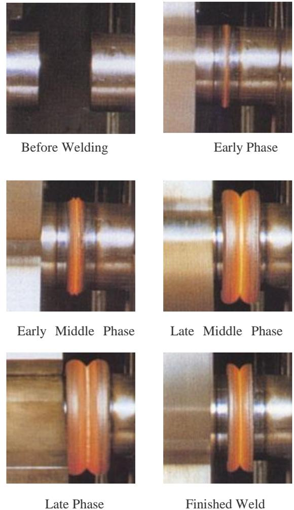
**Fig 1: Different phases of Friction welding processes**
