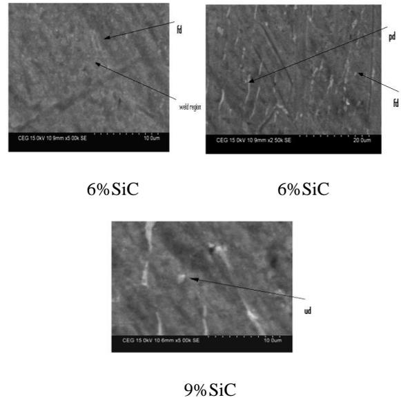
**Fig 3.3 microstructure analysis of Al7075/SiC 3%, 6%, 9 %**
