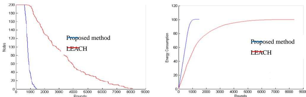
Fig 4. Number of alive sensor nodes      Fig 5. Energy consumption of sensor nodes
