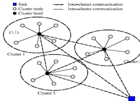
Fig. 2 Architecture of Clustering in WSN
